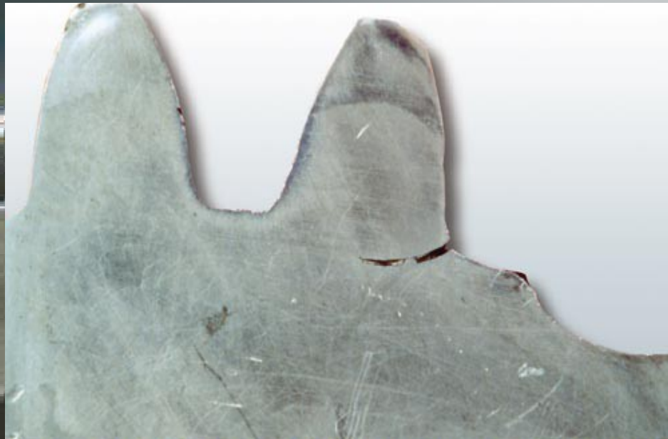
Figure 3. Fatigue Crack in Gear Tooth Root Fillet.
